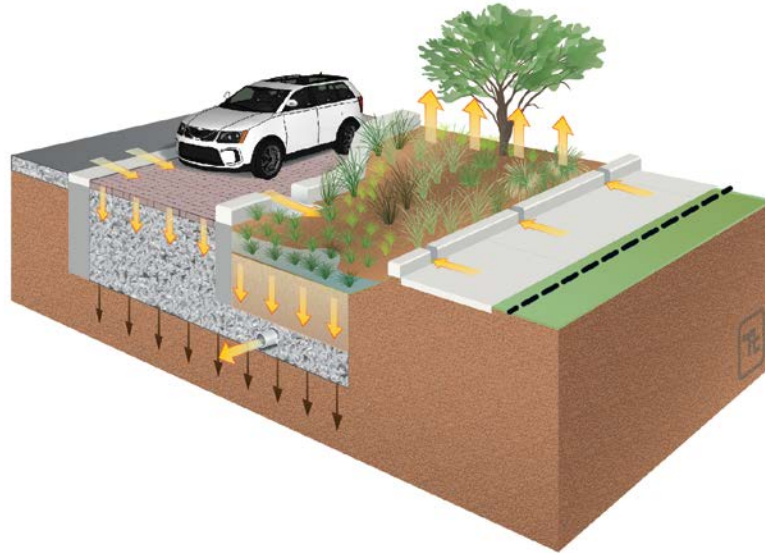
Figure 5-3. Conceptual schematic of green street/green infrastructure (arrows indicate water pathways)
